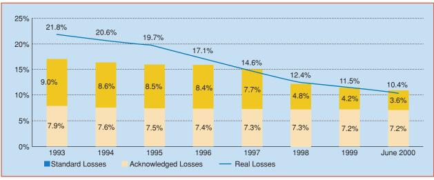
figure 16. Reduction of distribution losses.
