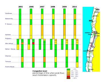
Figure 4. Congestions levels expected in the SIC Trunk system (2005 – 2010).
