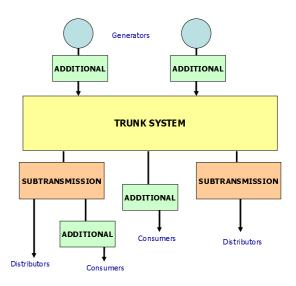
Figure 5 – Transmission segments under the new law.
