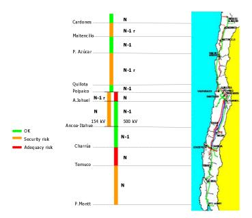
Figure 3. SIC Trunk system reliability status in 2004. All lines are 220 kV except Charrua-Ancoa-A.Jahuel 500 kV and Itahue-A.Jahuel 154 kV.
