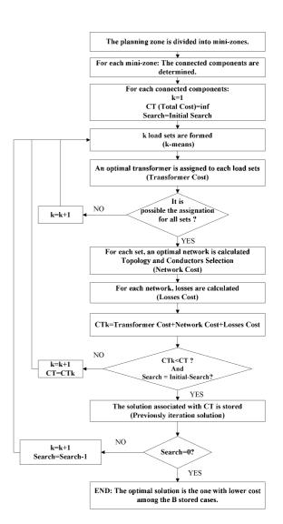
Fig. 2. Micro-optimization algorithm.
