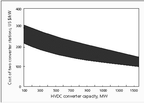
Fig. 3. Cost of two converter stations [6]
