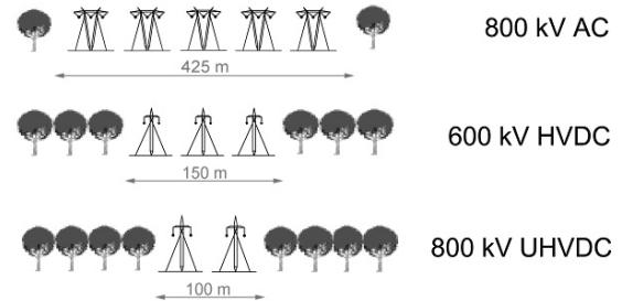
Fig. 2. Pilons needed to transmit 10 GW [5]
